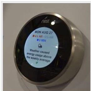
A Nest learning thermostat reporting on energy usage and local weather
