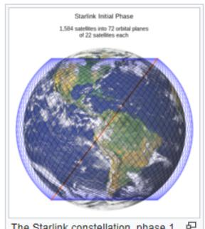
The Starlink constellation, phase 1, first orbital shell: 72 orbits with 22 each, therefore 1584 satellites at 550 km altitude
